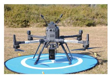
Figure 2: Lifeseeker UAS with sensor pod attached
