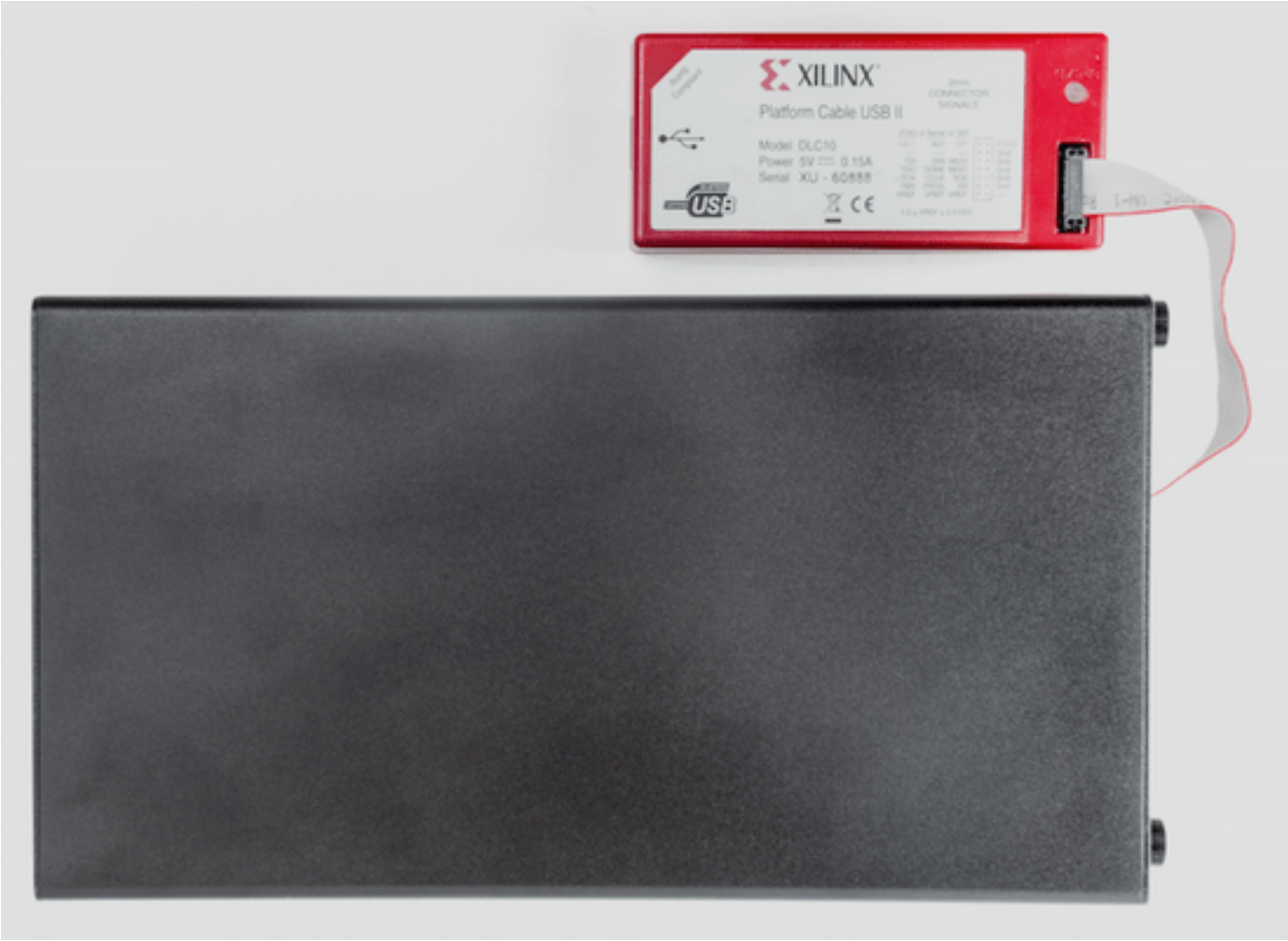
Figure 12: Thunderbolt 3 chassis closed up with Xilinx JTAG interface installed
