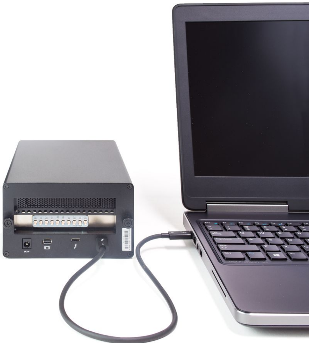
Figure 10: Sidekiq X4 & HTG-K800 FPGA host board installed into a Thunderbolt 3 chassis, interfaced to a laptop via a Thunderbolt 3 cable
