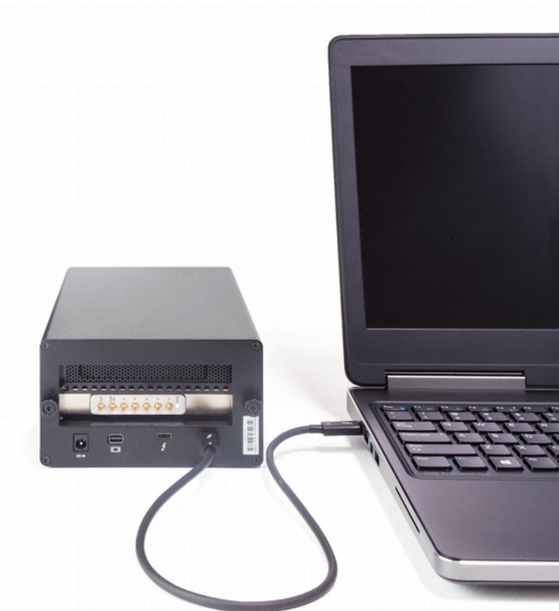
Figure 10: Sidekiq X2 + HTG-K800 FPGA host board installed into a Thunderbolt 3 chassis, interfaced to a laptop via a Thunderbolt 3 cable
