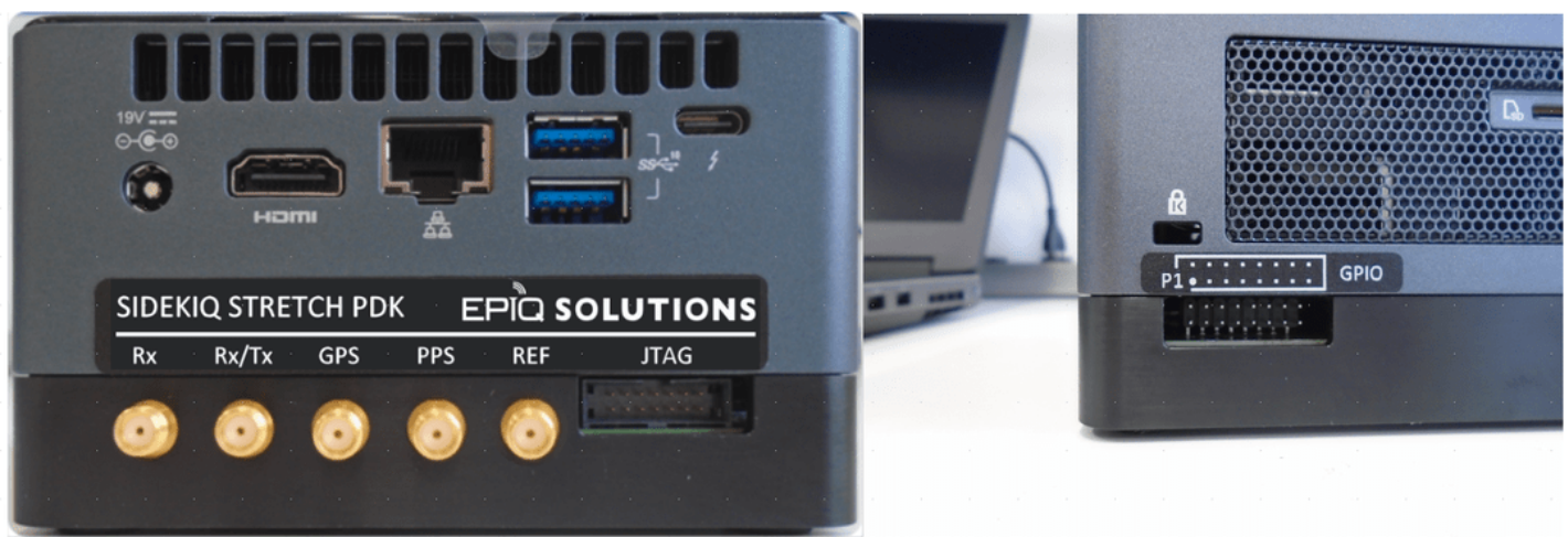
Figure 13: Sidekiq Stretch NUC hardware I/O interfaces
