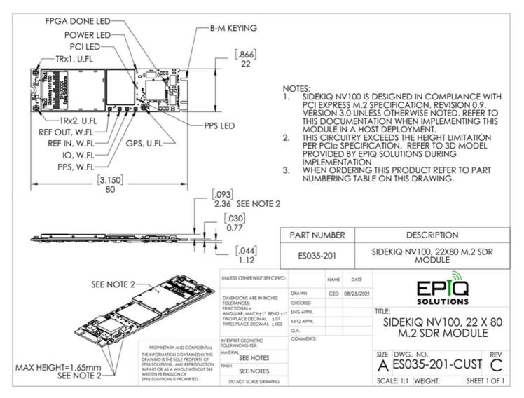
Figure 11: Sidekiq NV100 dimensioned drawing
