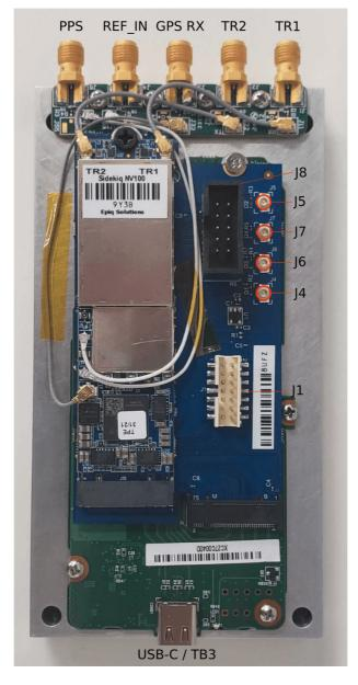
Figure 8: Sidekiq NV100 JTAG Fixture
