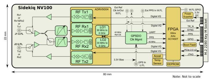
Figure 2: Sidekiq NV100 block diagram
