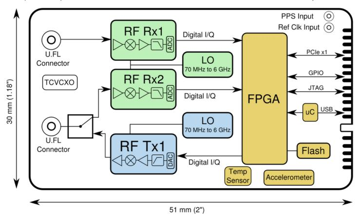
Figure 1: Block diagram of the Sidekiq MiniPCIe card
