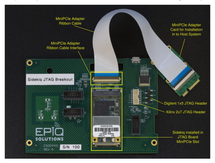
Figure 4: Sidekiq JTAG Board plus MiniPCIe adapter card for use in debugging
