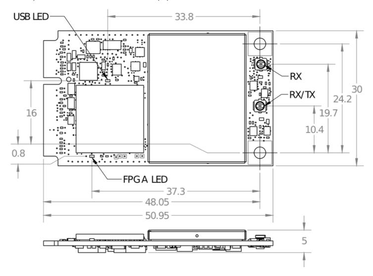
Figure 5: Sidekiq dimensioned drawing
