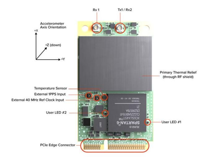
Figure 2: Annotated diagram of Sidekiq hardware I/O interfaces
