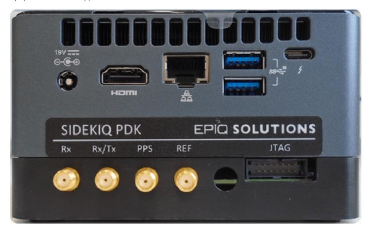
Figure 6: Sidekiq NUC hardware I/O interfaces
